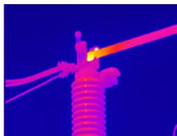
An alternative to Delta T calculations is a formula known as Tmax Corrected. This formula is based upon an IEEE formula and calculates pass/fail criteria based upon several factors including equipment type, ambient air temperature, and circuit load.
