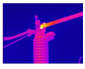
Perhaps the most common application for infrared thermography is PdM inspections of electrical distribution systems. However, in focusing on the inspection, many overlook the critical step of properly preparing for the
