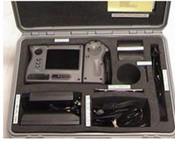
Nearly all thermal imagers are provided with compartmentalized carrying cases. These cases usually have die cut foam liners to protect the imager and its components and accessories. Labeling each compartment makes it easy to inventory compartments for the subject item(s). When labeling carrying case compartments, keep the following in mind:
